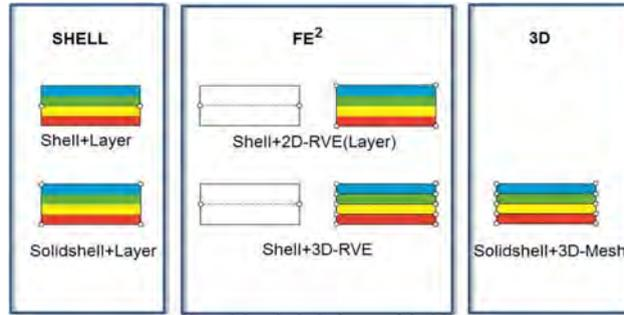
Fig. 1. Different discretization models for thin laminated structures.
