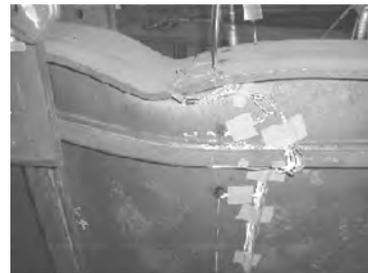
Fig. 1. Observed flange vertical buckling [2].
